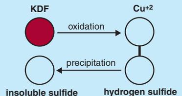
**KDF process media** converts hydrogen sulfide to insoluble sulfide, which can be removed by backwashing.
