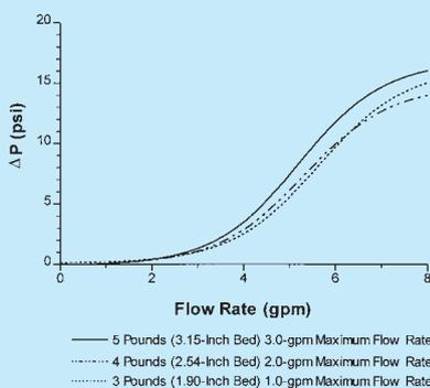
Maximum Flow Rate for 95% Reduction as a Function of the Amount of Medium
