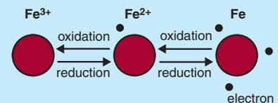
**KDF process media** act as catalysts to change soluble ferrous cations into insoluble ferric hydroxide, which is easily removed by regular backwashing.
