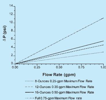
Maximum Flow Rate for 95% Reduction as a Function of the Amount of Medium
